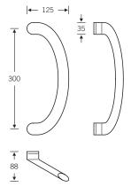
The flattened oval pull handle series 6533, 6534, 6535 and 6536 see FSB's philosophy of the ovally gripping hand and the diagonal moving arm put to effect in telling manner. The circular fastening section has been shortened and the grip tilted
