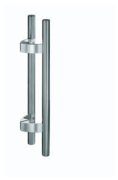
FSB has supplemented its proven and long-successful in-line pull series in aluminum and stainless steel with a particularly safe-to-grip design featuring heavily offset fastening points on which the ends of brackets are incorporated into the pull section. The in-line pull sections are supplied with a diameter of 35 mm in either aluminum or stainless steel. The brackets are made of aluminum and anodized in the metal's natural color.
